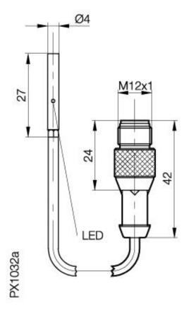
**Inductive Sensors** BES 516-3017-G-E4-C-S 4-00,2 D4 x 27 normally-closed Sn=1,5mm shielded
